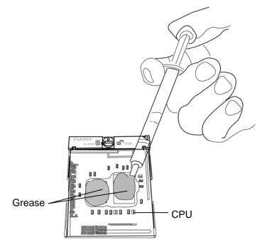
Figure 4-35 Applying new grease
